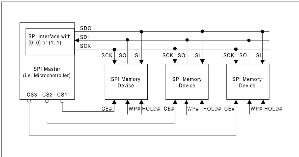
Note: 1. The Write Protect (WP#) and Hold (HOLD#) signals should be driven, High or Low as appropriate.
